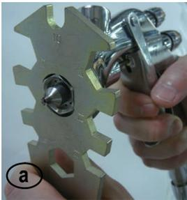
a. Disassembly fluid nozzle (2-1),
